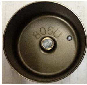
Figure 1: .3173” (8.06MM) Intake Lifter
